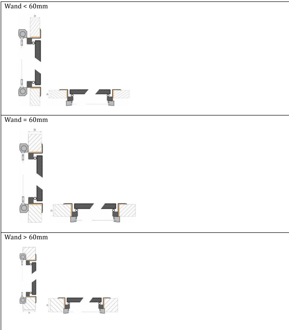
Figure 2 Mounting options for windows in different wall thicknesses
