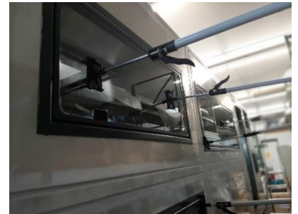
Figure 6 Supporting clips to fix the window during the drying process.
